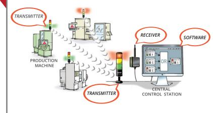
Our Machine Monitoring Smart Solution is the perfect combination of a signal device, wireless technology and an ingenious software package. The common interface on all machines, equipment and workstations is the signal tower. The transmitter has a transmission range of up to 300m clear line of sight. Range can be extended to up to 900m with a repeater.
