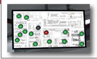
Client has a facility plant with 120 stations in use. Their aim is to track downtime on machines and systems. Signal tower lights are customized to report stop and downtimes.
