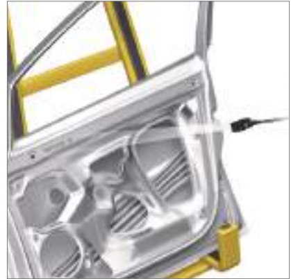
Reading lot numbers and codes on automotive body parts
