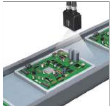
Identification of electronic components
