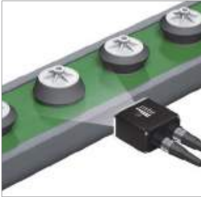
Orientation inspection of attached rubber
