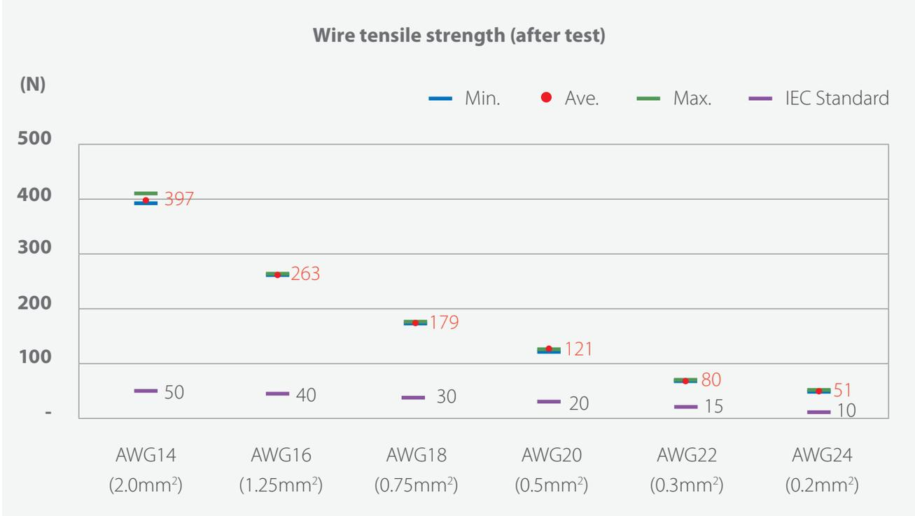
As tested by Omron in December 2015. Value with solid wire, Value after test is measured after leaving 96 hours in atmosphere at 105°C.
