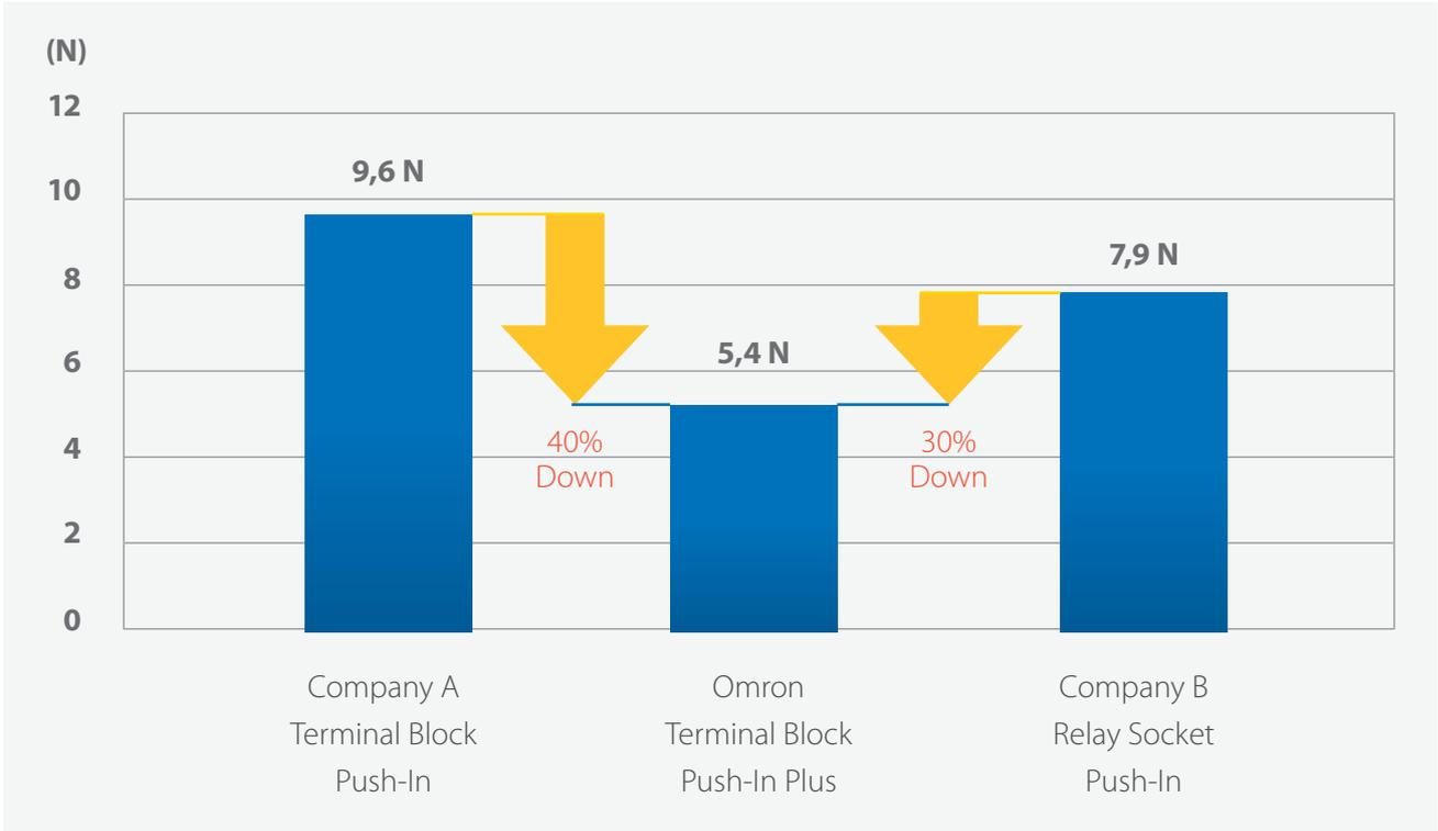
Measurement with steel gauge supposing AWG20 (0.5mm<sup>2</sup>) solid wire.
